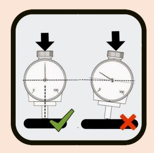
We are distributing Shore Meter A and all the discussions and descriptions are about them only. Higher numbers on the scale indicate a greater resistance to indentation and thus harder materials. Lower numbers indicate less resistance and softer materials. Durometer measurement scales range from 0 to 100 and simply represent a relative comparison of hardness difference.
